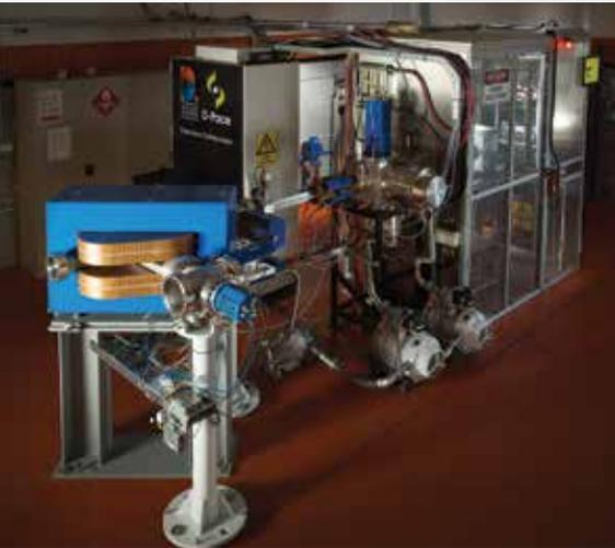
The Ion Source Test Facility is located at Buckley Systems Ltd (BSL), in Auckland, New Zealand. A joint project owned by Canadian company D-Pace, Inc., and BSL, the facility was conceived, designed, and partially built at D-Pace's location in Nelson, BC. BSL manufactured the hardware and D-Pace staff assembled and integrated the system in Auckland, with support from BSL staff. The facility has been operational since March 2016.
